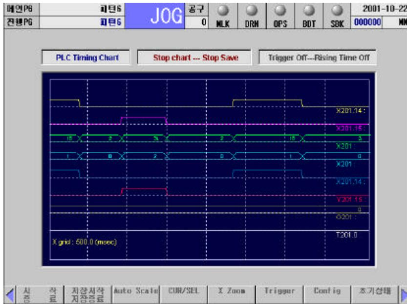
PLC ON/OFF Bit Timing Data
